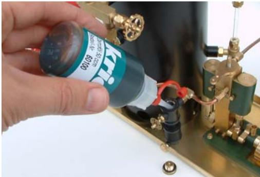
Before oil can be filled into the lubricator, the condensed water of the former running inside the lubricator has to be let out. For this reason open both screws of the lubricator and put some paper towel underneath. Now some drops of condensed water will come out. Now you can fill up the lubricator with special steam oil (Order No. 60100). Close the lower nut when oil is intending to come out at the bottom.
